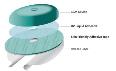
Patented UV curable adhesives provide water resistant bonding and low to no residual monomer after cure.
